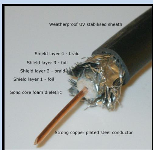
For optimum signal transfer, all coaxial cable in a digital TV antenna system should meet the RG6Q specification. Any cable that does will have RG6Q printed on it at 1 meter intervals.
