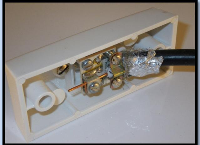
b. In order to connect the coaxial antenna cable to the back of the socket, it is necessary to strip back the cable shielding to expose the centre conductor. This creates a break in the cable shielding, and can also affect the impedance\* of the cable. This is another point where unwanted signal noise can degrade your TV reception.
